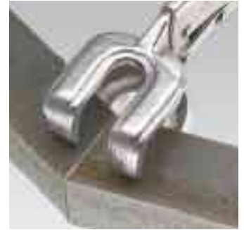
Secure fixing of metal section material for welding
