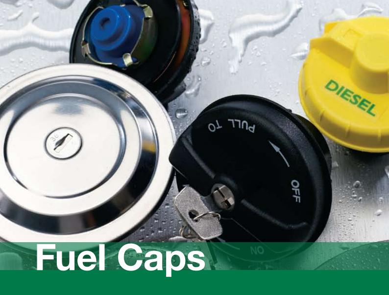
Tridon fuel caps are manufactured using either metal or plastic design suitable for use on sealed (non vented) or open (vented) fuel systems, and are available in both locking and non-locking options in various styles including metal bayonet, plastic screw and push and turn designs.
